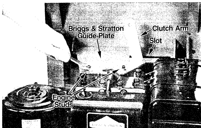
(Photo 8) Position the 8HP Briggs & Stratton Clutch Arm Guide-Plate as above. Plate holes nearest engine go over the two vertical engine studs. Secure the guide-plate to the studs with two locknuts. Other end of guide-plate will be connected later to handlebar.
