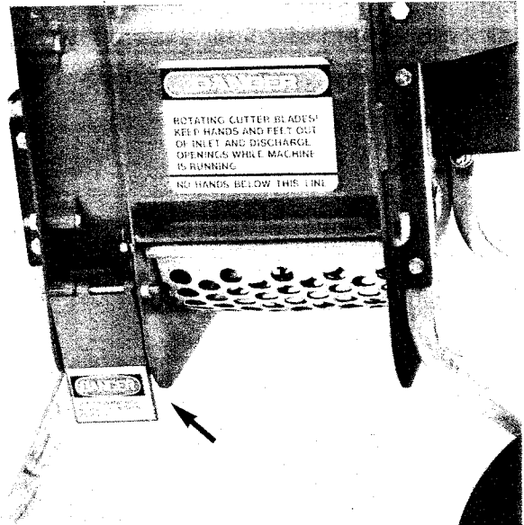
(Photo 24) Chipped materials exit from the Chipper Discharge Door shown above. Keep hands away!
