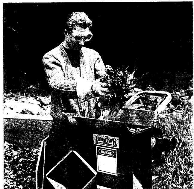
(Photo 35) Just drop loose material into the hopper.
